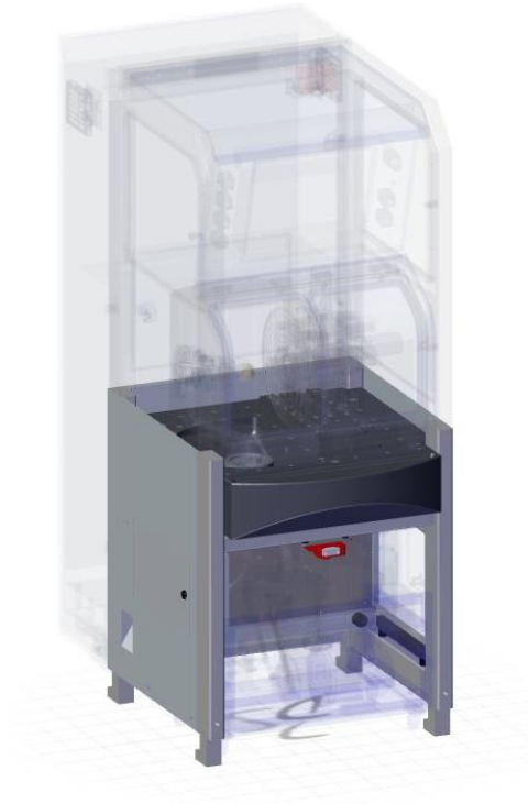
Figure 1: Polymer Granite Base & Welded Steel Frame
